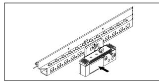
Fig. 6: Optional securing of the bracket
