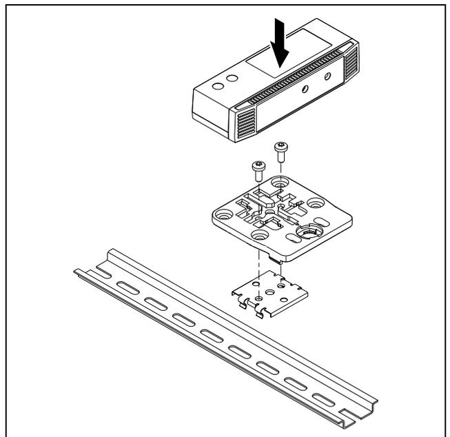
Fig. 8: Fastening the bracket to the spring clip
