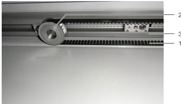
Fig. 35: Toothed-belt guide on the guide pulley
