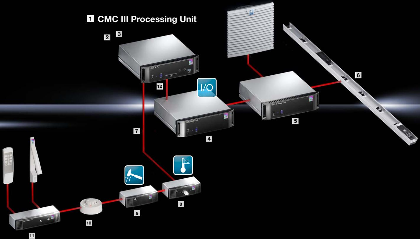
Computer Multi Control (CMC) is an alarm system for network and server enclosures, standard enclosures, containers and rooms.
