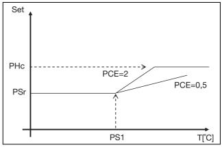
Fig. 39: Operating mode 2 – Relative (room temperature-based control **with** limit values)
