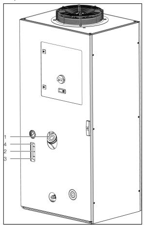
Fig. 32: Filling the cooling medium (shown 3335.790)
