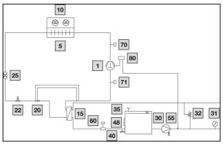
Fig. 9: Schematic diagram of chiller 3335.790, 3335.830, 3335.840, 3335.850, 3335.860, 3335.870
