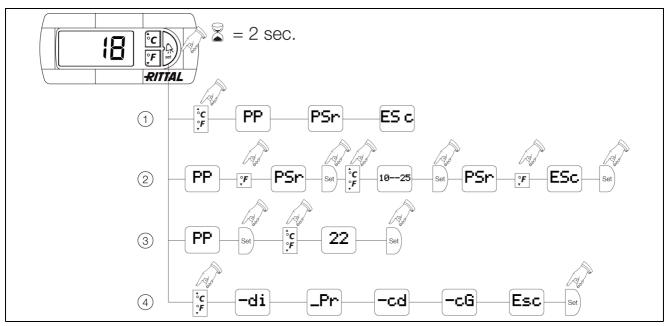
Fig. 37: Basic and customer level
