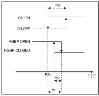
Fig. 44: Circuit for the HGBP valve
