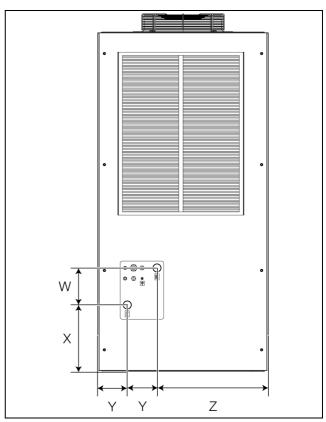
Fig. 24: Dimensions (supply connections) of rear excluding base/plinth (shown 3335.790)
