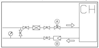
Fig. 26: Installation example with non-return and magnetic valve
