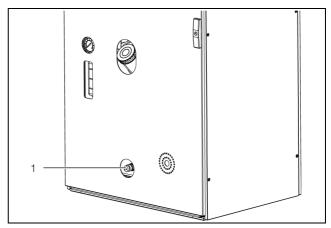
Fig. 48: Draining the tank
