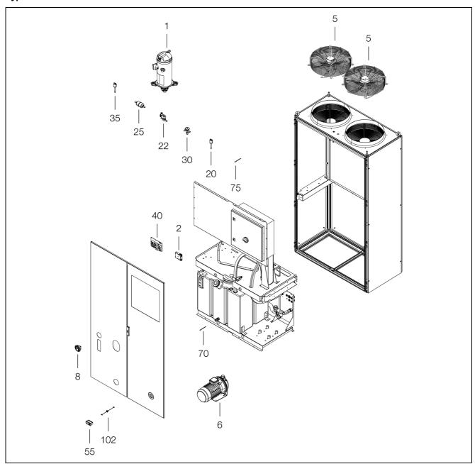
Fig. 104: Spare parts drawing for types 3335.860 and 3335.870
