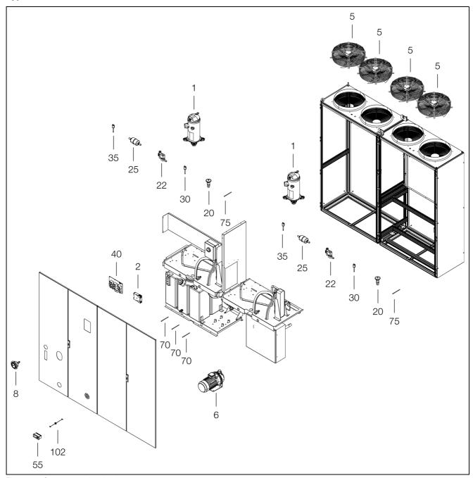
Fig. 106: Spare parts drawing for type 3335.890
