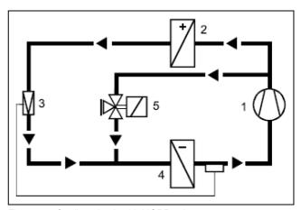
Fig. 43: Cooling circuit with HGBP valve
