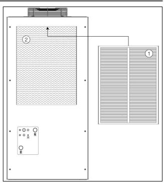
Fig. 31: Installation of the air filter
