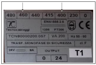
Fig. 29: Transformer connection
