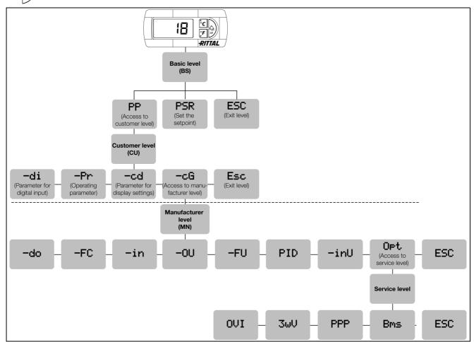
Fig. 36: Overview of programming levels
