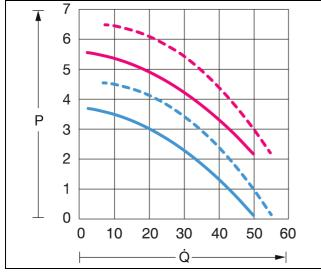
Fig. 11: Characteristic curve 3335.790 and 3335.830
