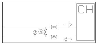
Fig. 28: Installation example with overflow valve
