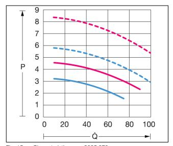
Fig. 15: Characteristic curve 3335.870
