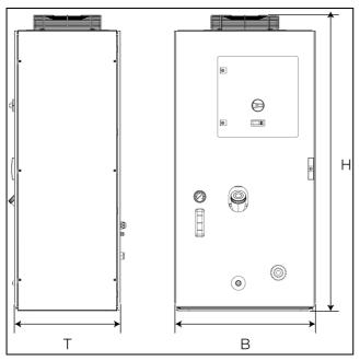
Fig. 23: Dimensions of front excluding base/plinth (shown 3335.790)
