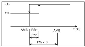
Fig. 40: Operating mode 3 – Relative (room temperature-based control **without** limit values)
