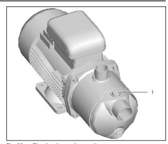
Fig. 33: Bleeding the cooling medium pump
