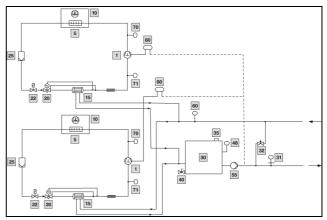
Fig. 10: Schematic diagram of chiller 3335.880, 3335.890
