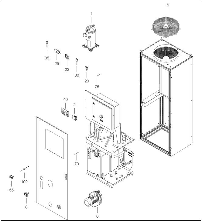
Fig. 103: Spare parts drawing for types 3335.790, 3335.830, 3335.840, 3335.850
