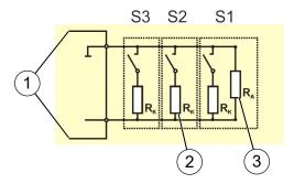
Fig. 53: Manual call points parallel connected
