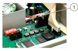
The replacement of the battery "control card CPU3" (Fig. 73/1) must be reported.
