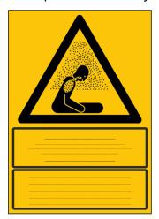
Fig. 2: Marking of the extinguishing zone (example)
