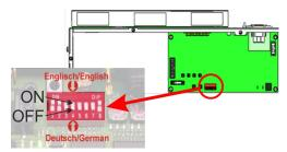
The system can communicate in "German" and "English". "German" is pre-set by the manufacturer but can be changed to "English" via a DIP switch (Fig. 27). Proceed as follows to make the changeover:
