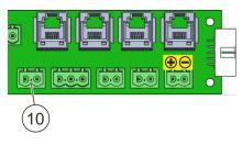
Fig. 41: Connection external alarm device
