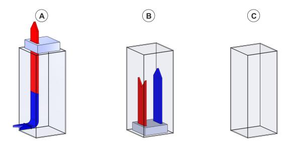
Fig. 18: Cooling air circuit 19" cabinet
