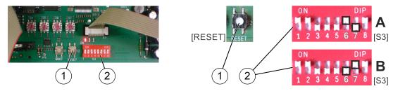
Fig. 49: [Reset] button and DIP switch "S3"
