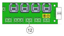
Fig. 52: Connecting terminal "Manual call point"
