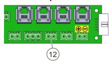
Fig. 14: Manual call point connection
