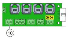
Fig. 12: Connection of external alarm device
