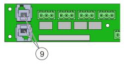
Fig. 17: Connection for networking
