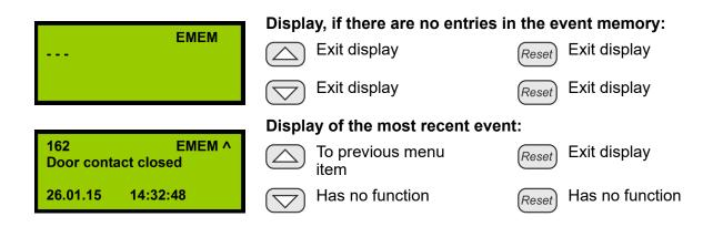
With activation of this control function "Review the event memory", the temporally most recent message is always displayed. It is possible to change to older messages using the [Up] arrow button. The symbol  $\Lambda$  in the upper right of the display shows that there are older messages present.
