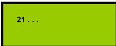
The current values are determined. The value displayed counts up to 64 (progress bar). No further operation is possible at this stage.
