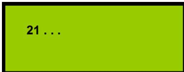
The current values are determined. The value indicated counts up to approx. 76 (progress bar). No further operation is possible at this stage.
