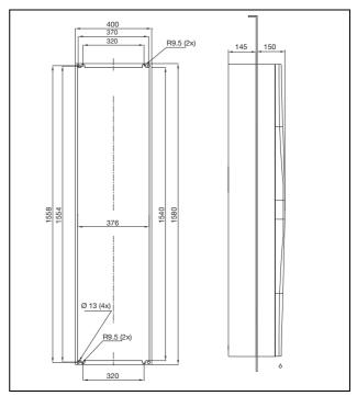
Fig. 103: 3328.xxx, 3329.xxx partial internal mounting
