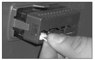
Fig. 39: Disconnect the connector from the display (2)
