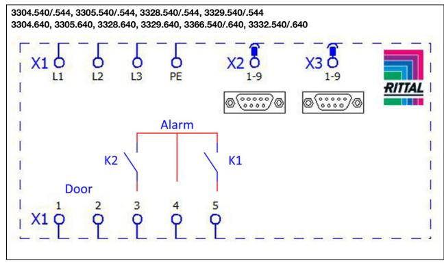
Fig. 25: Electrical wiring plan no. 3
