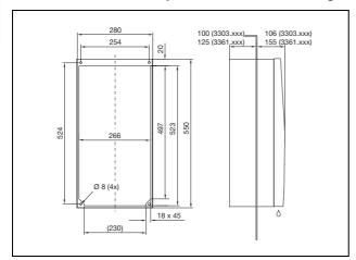
Fig. 101: 3303.xxx, 3361.xxx partial internal mounting
