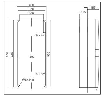
Fig. 102: 3304.xxx, 3305.xxx partial internal mounting
