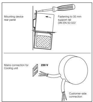
Fig. 20: Mounting external transformer (3361.x40 only)
