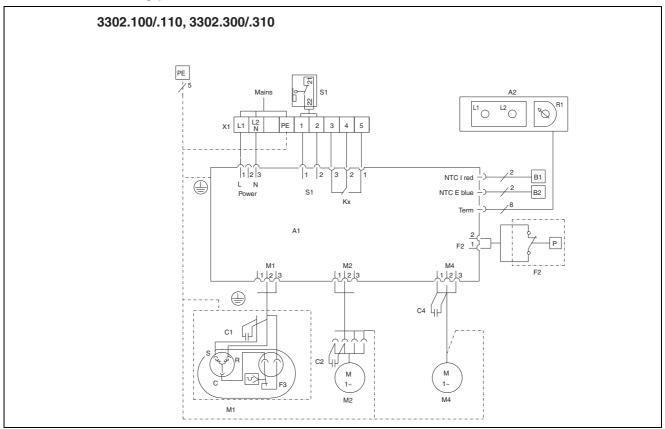
Fig. 111: Electrical wiring plan no. 1
