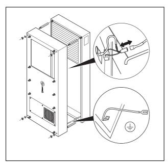
Fig. 11: Removing the cover
