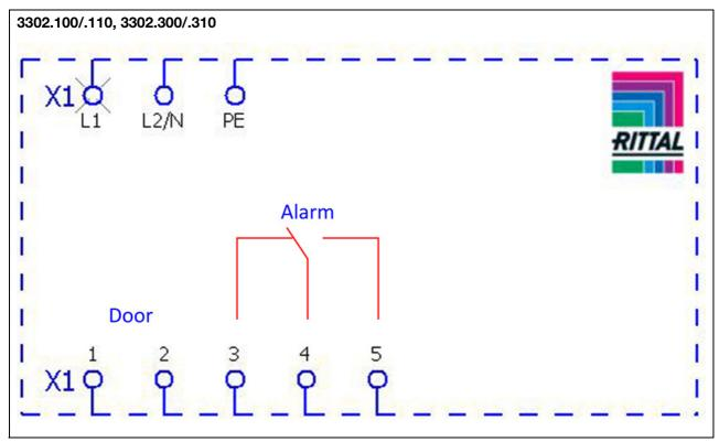
Fig. 23: Electrical wiring plan no. 1
