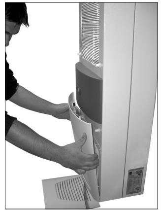
Fig. 36: Remove the bottom louvred grille
