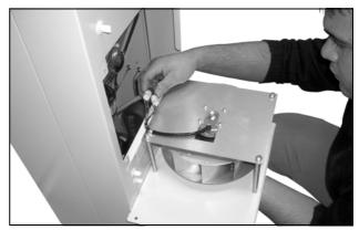
Fig. 65: Disconnect the fan connectors (1)
