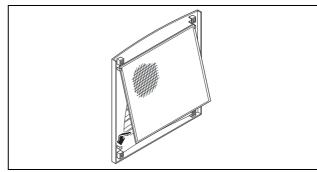
Fig. 26: Installing the filter mat
