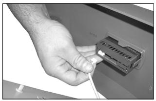
Fig. 60: Disconnect the display cable
