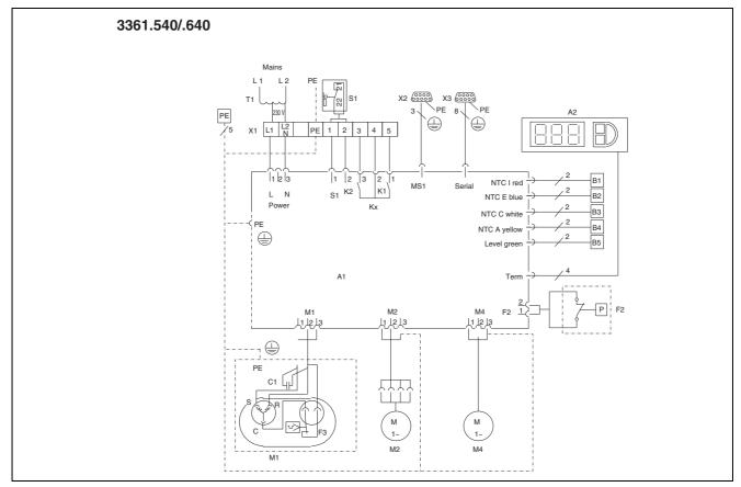
Fig. 113: Electrical wiring plan no. 3
