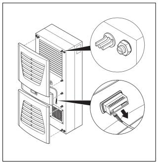
Fig. 15: Removing the louvred grille & disconnecting the display
