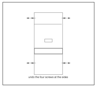
Fig. 79: Remove the cover (1)
