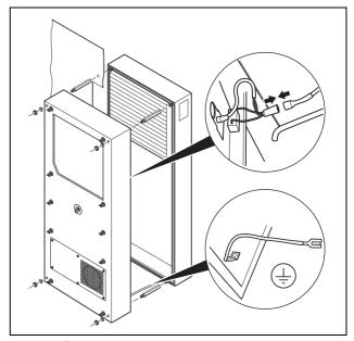
Fig. 13: Securing the cooling unit
