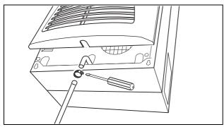
Fig. 19: Connecting the condensate discharge
