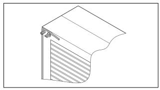
Fig. 16: Applying the self-adhesive tape
