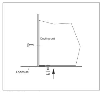
Fig. 78: Device mounting
