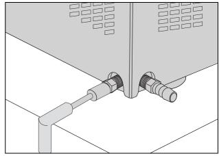
Fig. 9: Connecting the condensate discharge
