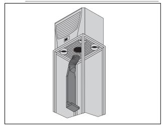
Fig. 4: Targeted air routing inside the enclosure
