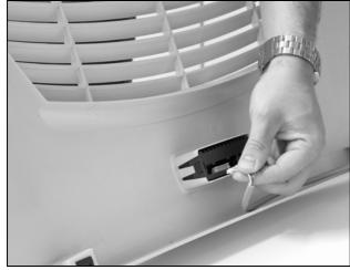
Fig. 24: Disconnect the connector from the display
