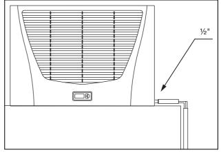
Fig. 10: Laying the condensate discharge
