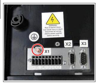
Fig. 11: Connection point, potential equalisation
