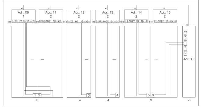
Fig. 13: Connection example: Door limit switch and master-slave operation
