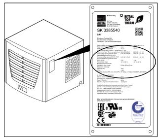
Fig. 32: Rating plate (technical data)
