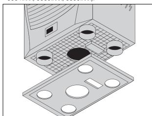
Fig. 7: Sealing plate underneath the plastic base of the cooling unit
