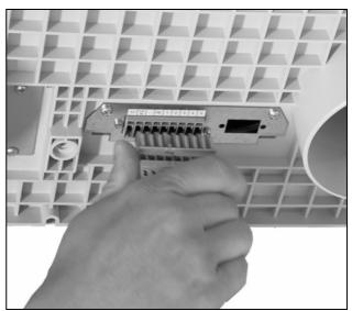
Fig. 21: Disconnect the mains plug
