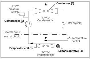
Fig. 2: Cooling circuit
