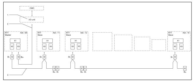
Fig. 12: Connection example: Master-slave operation
