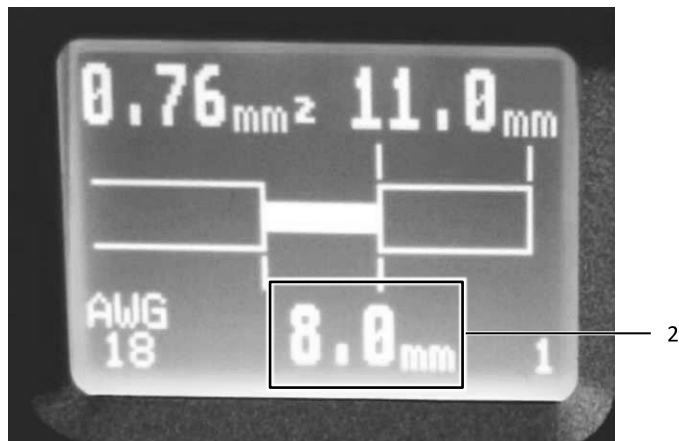
Fig. 6: Draw-off length in the display
