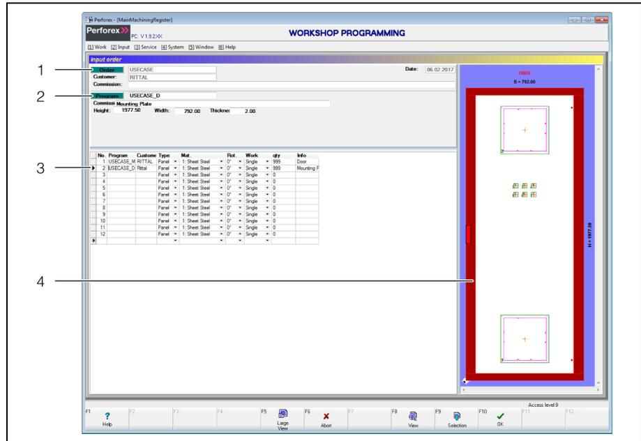
Fig. 35: "Order input" screen page with inserted raw panels
