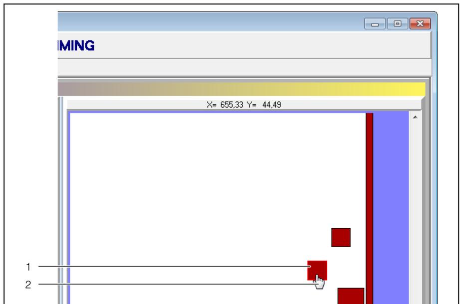
Fig. 8: Moving a blocked surface with the mouse
