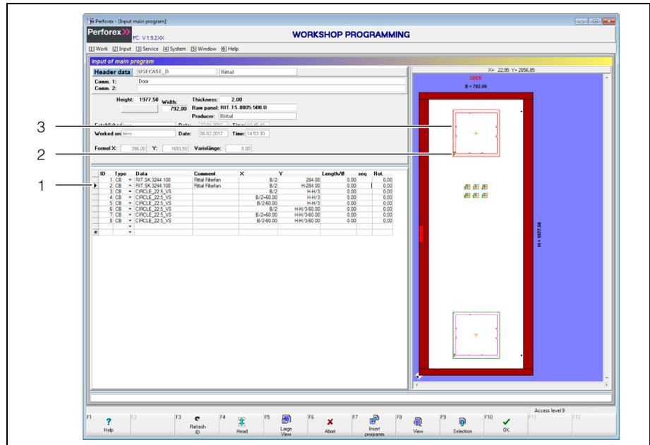
Fig. 9: Selected component part in the line data and the graphical representation
