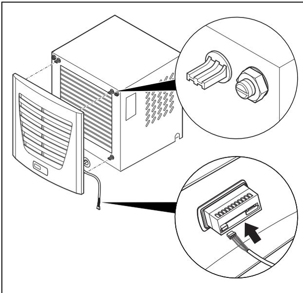
Fig. 16: Conectar o display e colocar as grades
