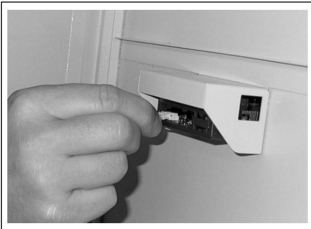
Fig. 13: Connect the display connection cable
