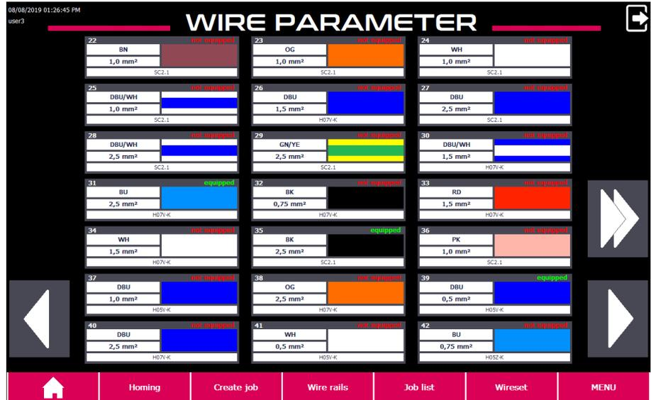
Wire parameters can be viewed, changed, deleted and copied as well as new wires created in this menu.
