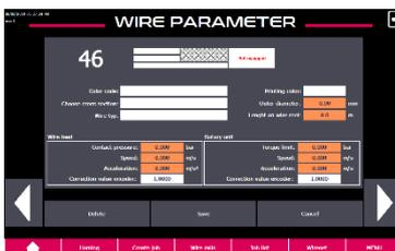
To reach the submenu in which the wire parameters can be entered or changed, select a wire parameter set.
