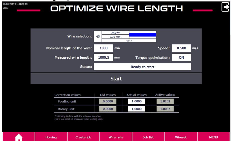
For each wire, slip occurs between the driven feed rollers of the wire feeder unit or rotary unit and the wire to be moved. Due to the resulting position error, the length by which a wire is moved for each rotation of the feed roller does not exactly match the roller circumference.
