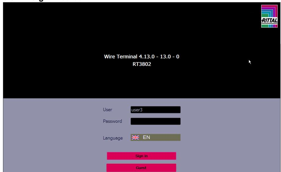
The sign-in screen is displayed immediately after the system startup. The upper half of the sign-in screen contains information about the installed software release of the system as well as the machine serial number. The lower half of the sign-in screen is used for the sign-in with user name and password (see section 3.3.10.13 "User administration") or as guest.
