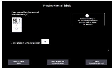
When a job is loaded, the pop-up window for the assignment of rails and the printing of rail labels opens. The rails are assigned automatically, provided appropriate rails have already been setup. The rail positions, however, can be overwritten manually. If no appropriate rail has been setup, an appropriate rail must be setup and the rail position made known.
