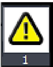
This symbol indicates pending or unacknowledged warning or error messages and is displayed in the foreground on each display page. If a new warning or error message becomes active, the message window opens automatically in the foreground. The window can be closed at any time with the "Close symbol" (X symbol) at the top right in the message window, even when the message has not yet been acknowledged. Tapping the "Messages symbol" reopens the window.
