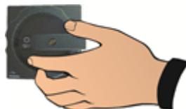
Turn the master switch on the enclosure of the Wire Terminal from the "ON/I" position (vertical) counter-clockwise to the "OFF/O" position (horizontal).
