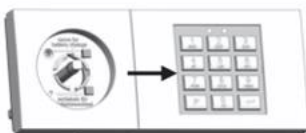
Fig. 4.4: Move the top part of the input unit in the direction of the arrow to the stop.
