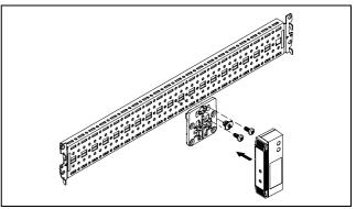
Fig. 8: Fastening the sensor to a system chassis
