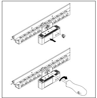
Fig. 6: Mounting the sensor in the enclosure or IT enclosure
