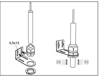
Fig. 2: Installing the sensor probe
