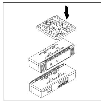
Fig. 4: Attaching the sensor to the bracket
