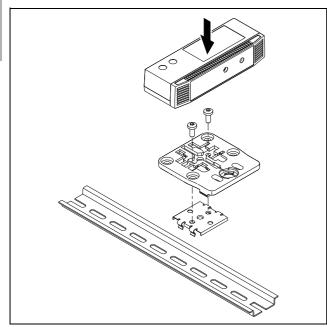
Fig. 9: Fastening the bracket to the spring clip
