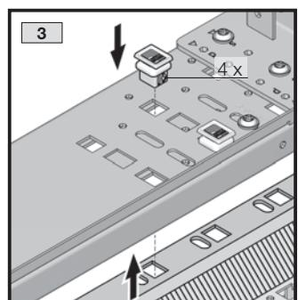
4.3 Montage Bürsten-Kit an Kabelkanal
