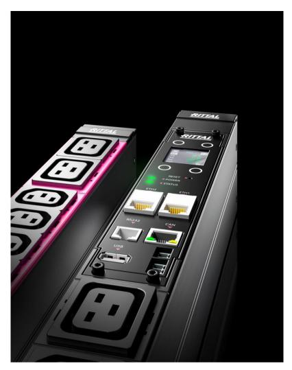
The core task of a PDU is to distribute energy, which is why they can be found in the A and B power supply on a redundant basis. Depending on their design, PDUs can monitor and switch the power supply down to the level of individual socket outlets, which also means these network-capable devices support remote maintenance.
