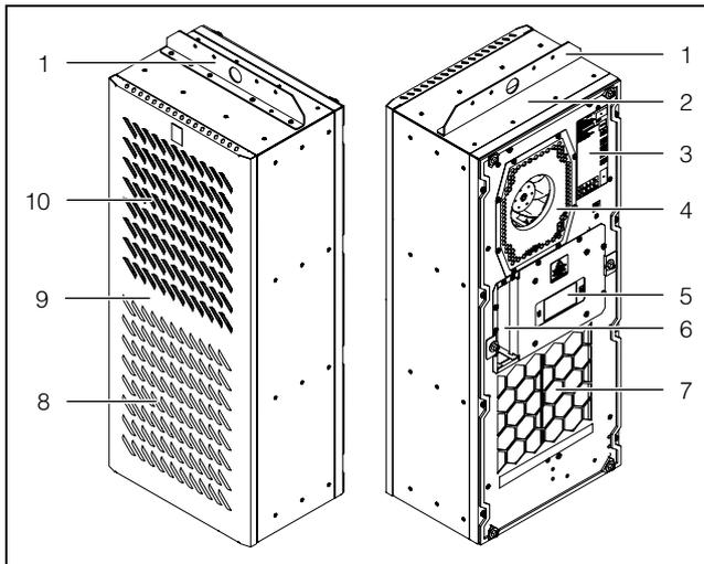
Fig. 2: Main components of cooling unit (SK 3185330)
