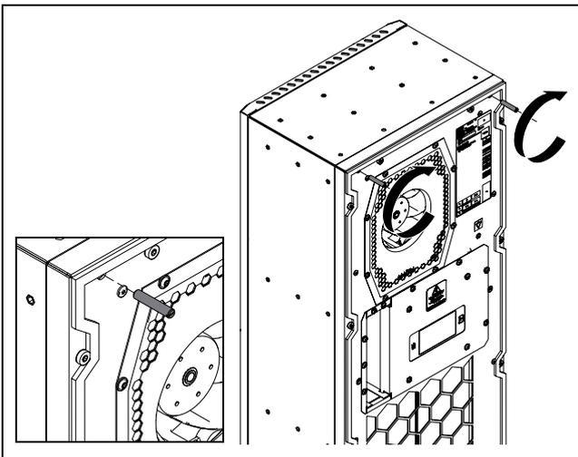
Fig. 12: Tighten the grub screws at the top
