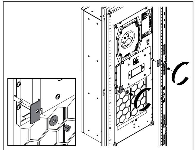
Fig. 18: Fit the central L-shaped brackets
