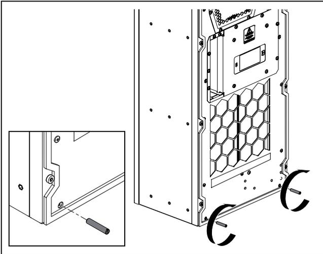
Fig. 11: Tighten the grub screws at the bottom
