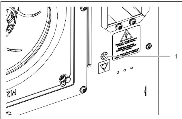
Fig. 34: Connection point for potential equalisation (example illustration)
