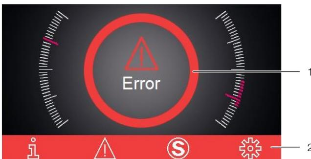
Fig. 44: Screen in the event of a malfunction
