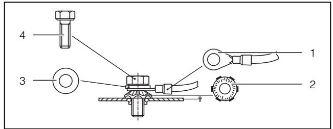
Fig. 35: Potential equalisation arrangement
