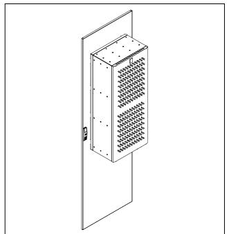
Fig. 8: Fitting without a mounting frame
