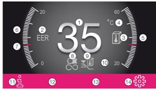
Fig. 41: Layout of the start screen
