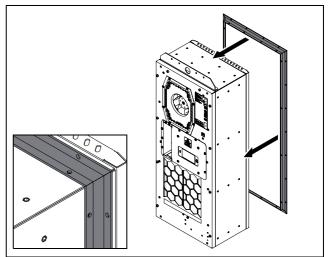
Fig. 21: Position the mounting frame
