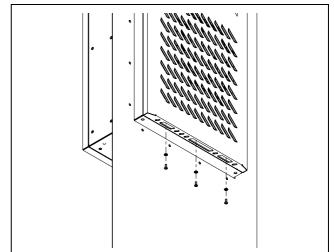
Fig. 27: Loosen the assembly screws
