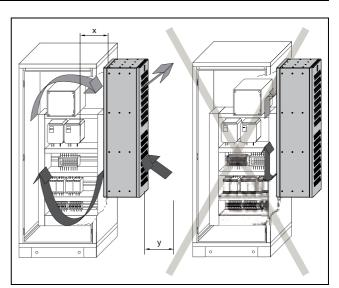
Fig. 6: Air circulation inside the enclosure
