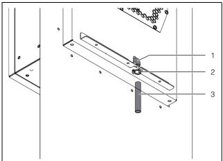
Fig. 30: Connection for condensate discharge hose
