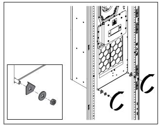
Fig. 15: Fit the bottom corner brackets
