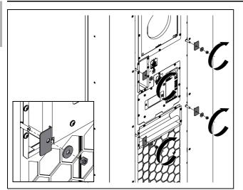
Fig. 19: Fit the central L-shaped brackets
