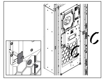
Fig. 18: Fit the central L-shaped brackets
