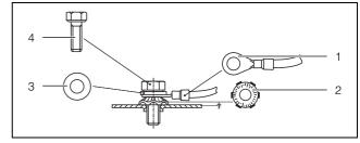
Fig. 35: Potential equalisation arrangement
