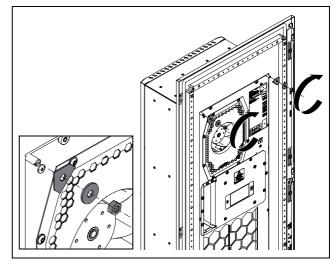
Fig. 14: Fit the top corner brackets
