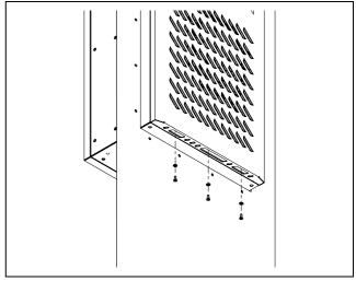
Fig. 47: Loosen the assembly screws
