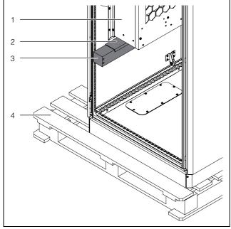
Fig. 5: Internal mounting of the shipping braces
