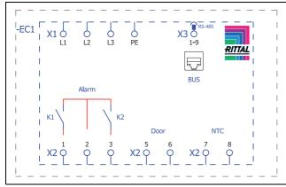
Fig. 38: Circuit diagram SK 3188340, SK 3189340
