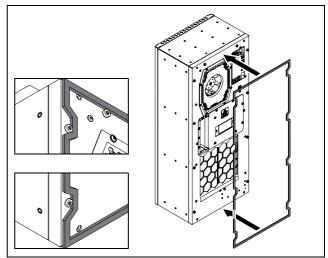
Fig. 10: Laying the seal
