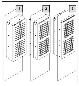
Fig. 9: Mounting options with a mounting frame
