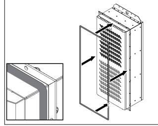
Fig. 24: Slide over the seal position
