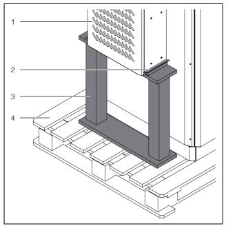
Fig. 4: External mounting of the shipping braces
