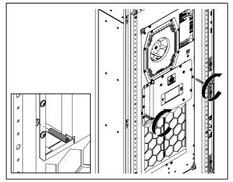
Fig. 16: Tighten the central grub screws
