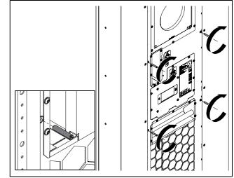
Fig. 17: Tighten the central grub screws
