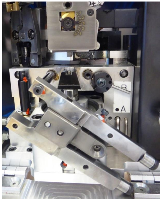
Fig. 25: Stranded wire fixing unit dismantled
