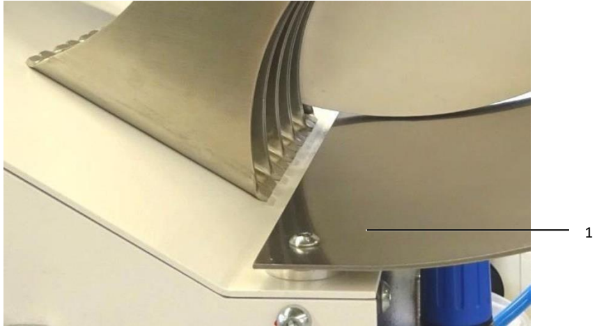
Fig. 5: Installed retaining plate
