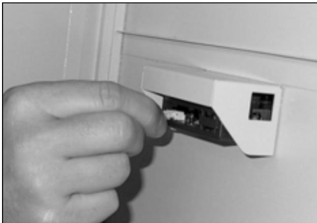
Fig. 15: Connect the display connection cable
