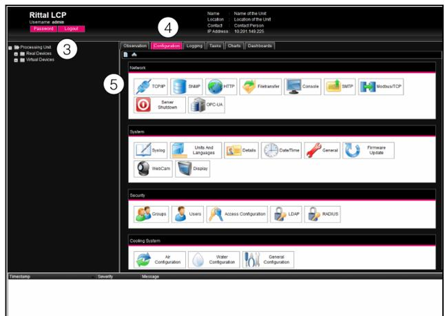
Fig. 90: Adjusting the TCP/IP settings
