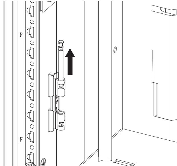
Fig. 51: Opening the hinge pins
