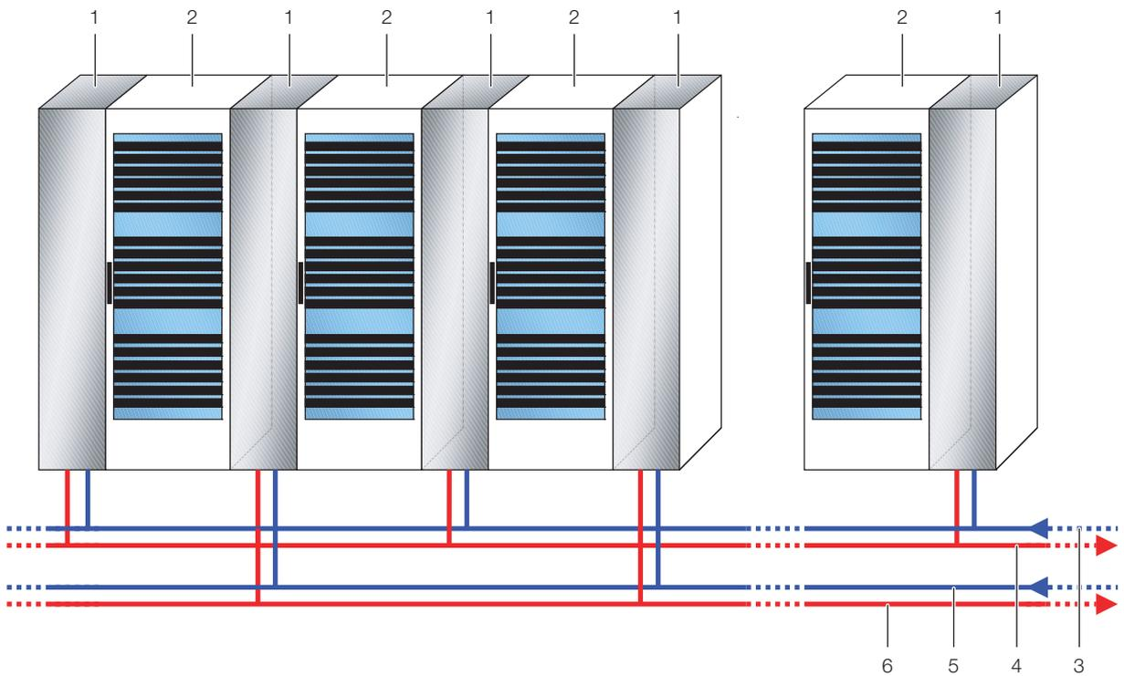
Fig. 19: Redundant cooling and double alternating water supply
