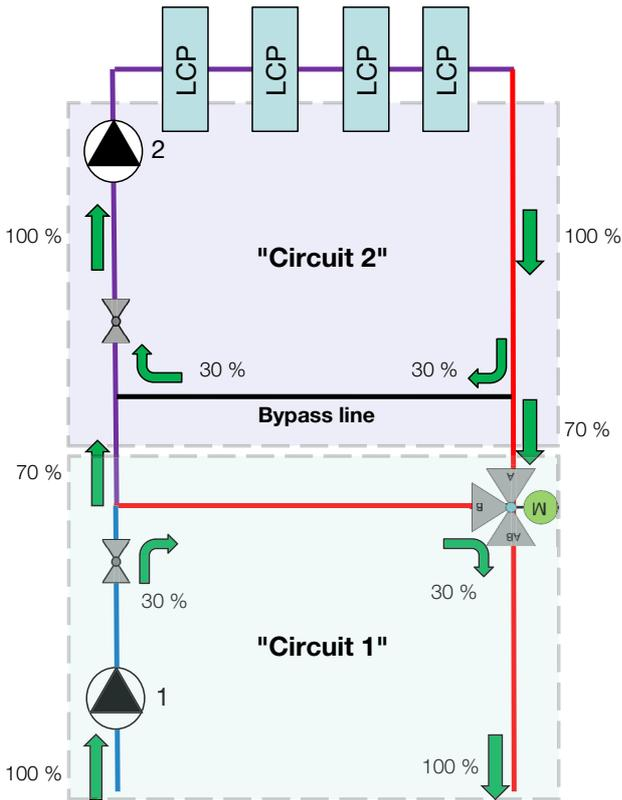
Fig. 83: Injection circuit (layout diagram)
