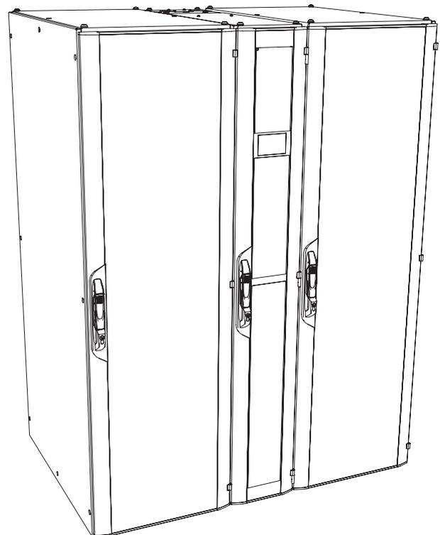
Fig. 8: LCP Rack on two server enclosures
