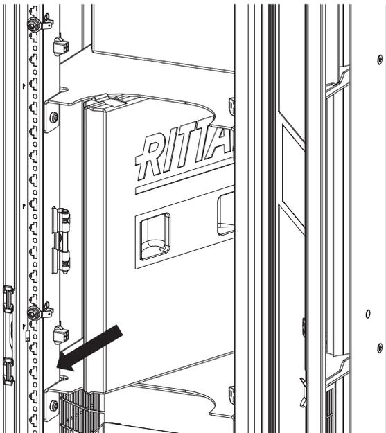
Fig. 50: Turned cover in the rack unit
