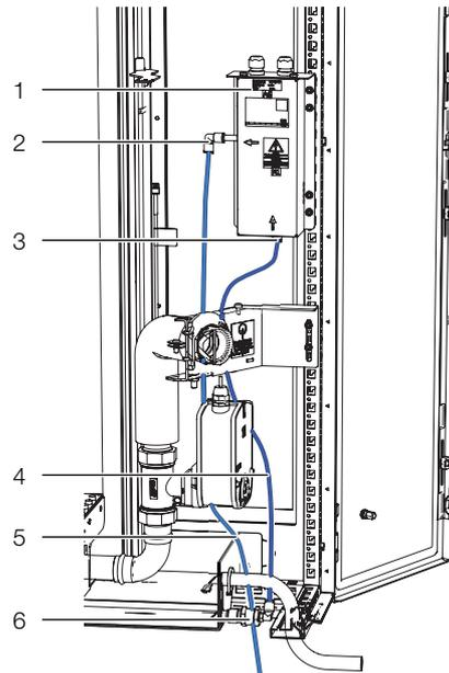
Fig. 61: Connecting the hoses to the LCP
