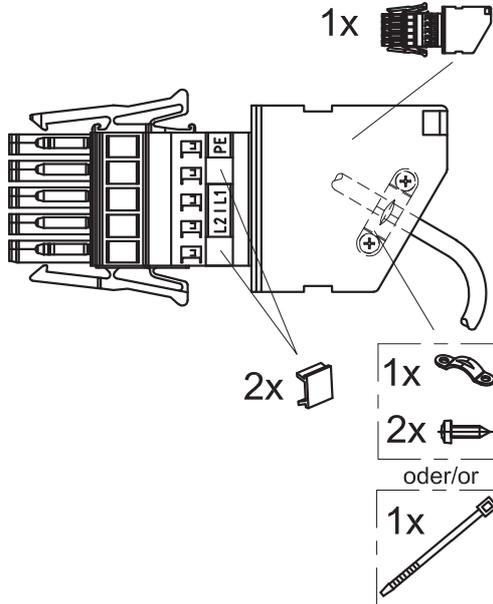
Fig. 77: Connector diagram for single-phase connection – NSA version
