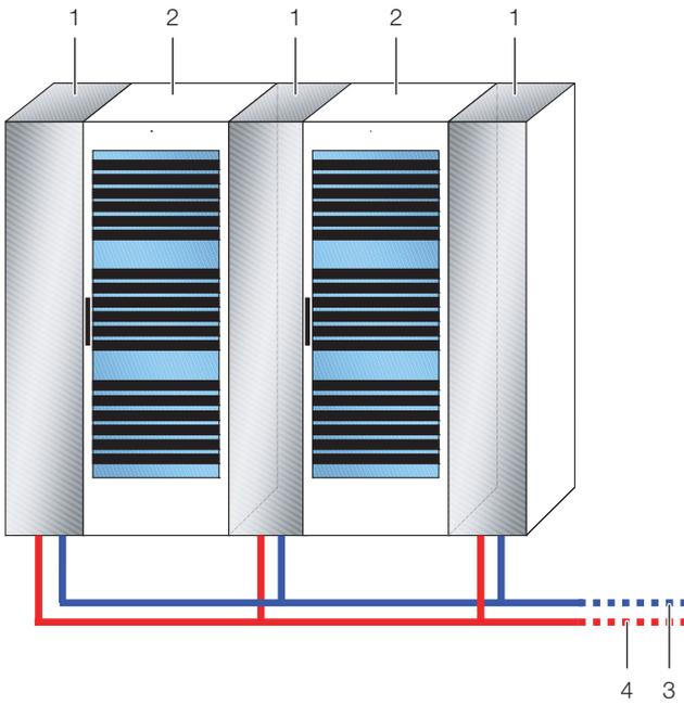
Fig. 18: Redundant cooling with three LCP Racks
