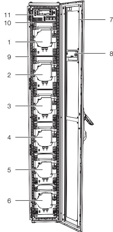
Fig. 13: Liquid Cooling Package front – open front door
