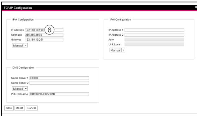
Fig. 91: Adjusting the TCP/IP settings
