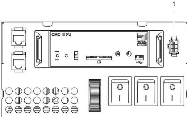
Fig. 57: Connection point at the electronic module
