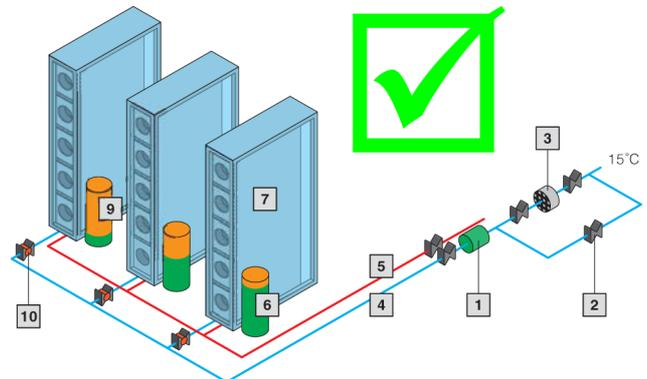
Fig. 85: Cooling distribution with hydraulic balancing
