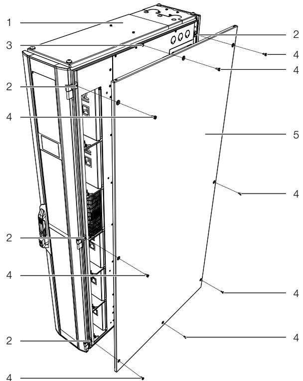
Fig. 41: Attach the side panel to the LCP
