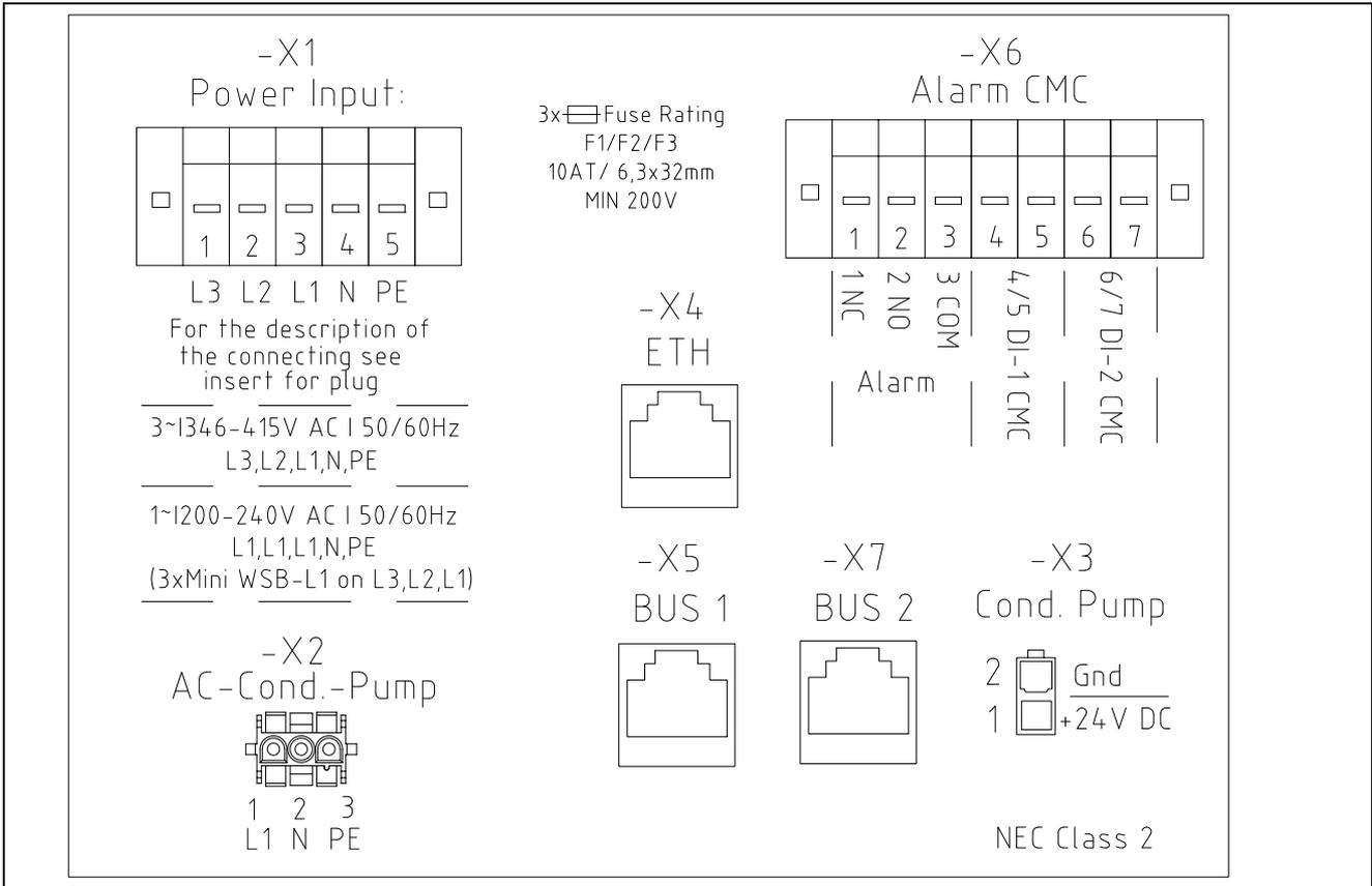
Fig. 128: Wiring diagram global version
