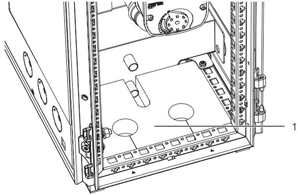
Fig. 25: LCP CW rear view – Space for inserting the connection hoses
