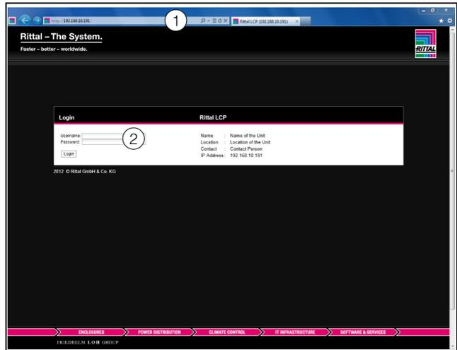
Fig. 89: Log-on screen with an HTTP connection
