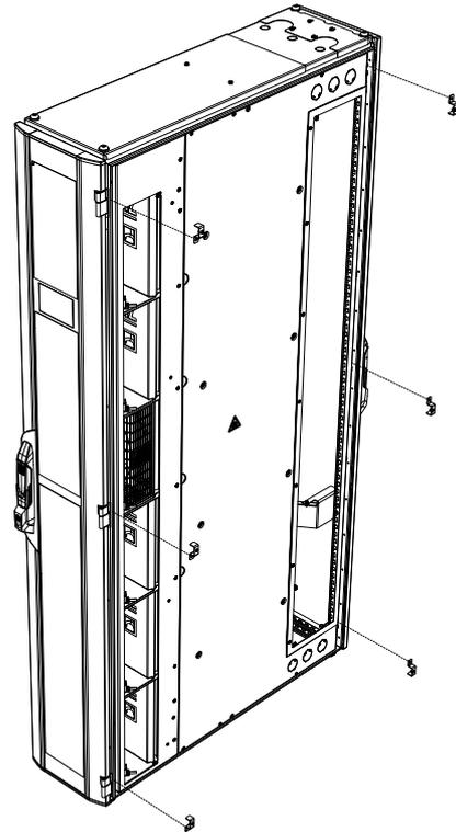
Fig. 40: Attach the brackets to the LCP
