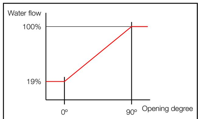
Fig. 4: Opening degree of the control valve
