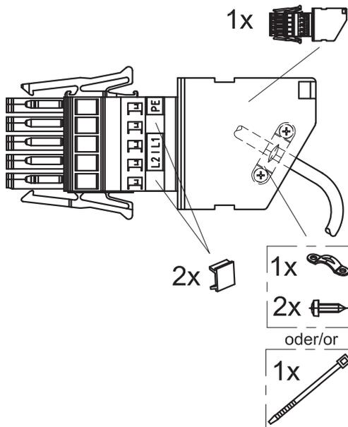
Fig. 78: Connector diagram for two-phase connection – NSA version
