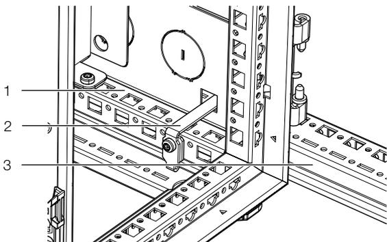
Fig. 36: Connection element in the rear area VX/TS
