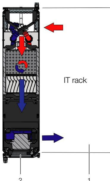
Fig. 134: "Front to back" cooling principle with bayed LCP Rack
