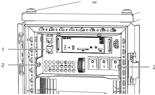
Fig. 26: Electronic module in the LCP
