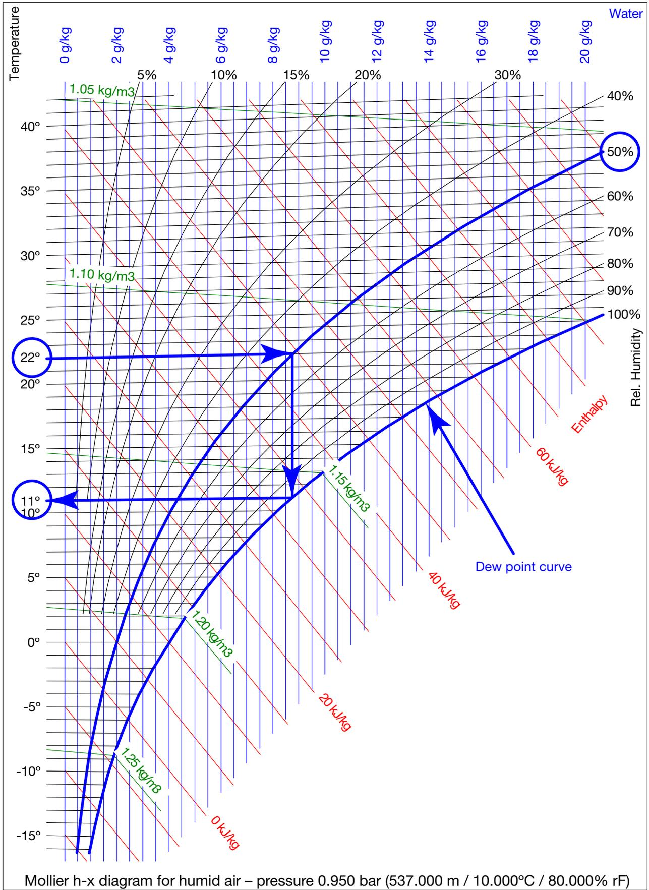
Fig. 6: Mollier h-x diagram for humid air
