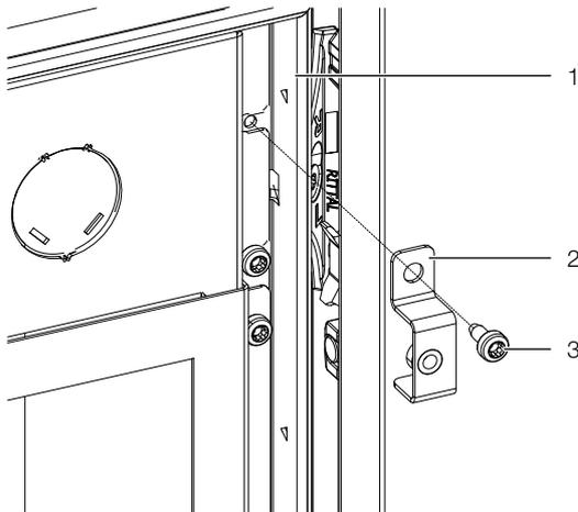
Fig. 39: Mounting bracket for attaching the side panel
