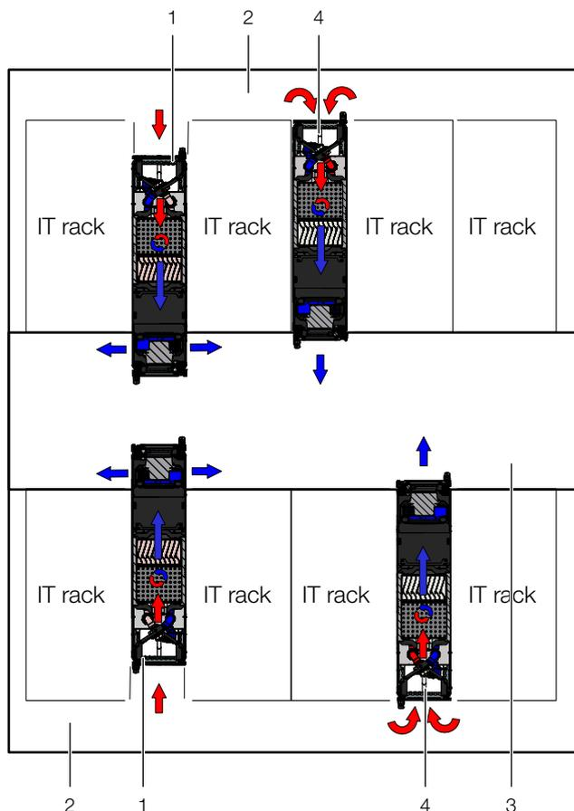
Fig. 27: Installation room with cold aisle compartmentalisation
