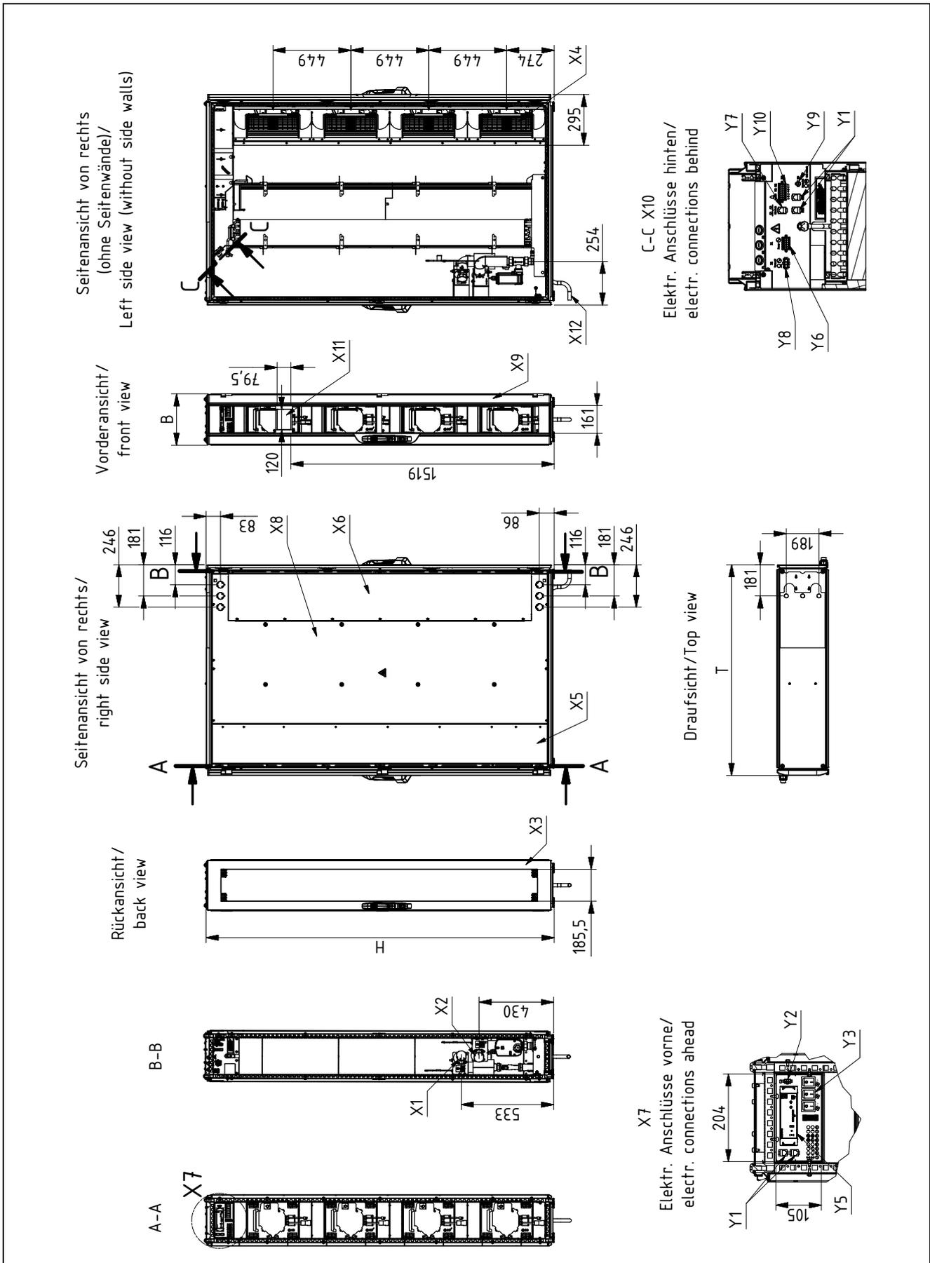
Fig. 126: Overview drawing of LCP Inline Flush, 30 kW
