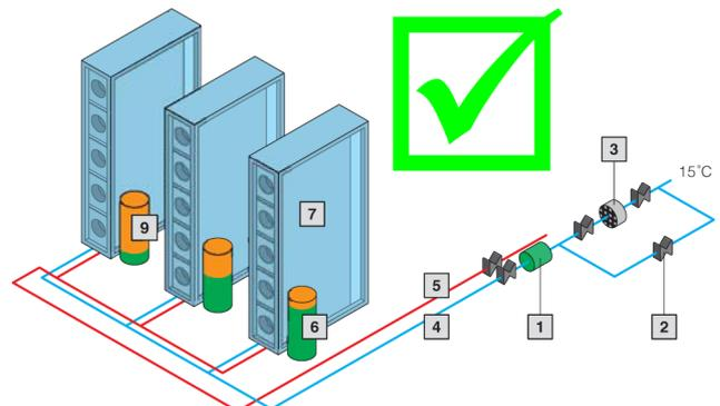
Fig. 86: Cooling distribution with Tichelmann principle
