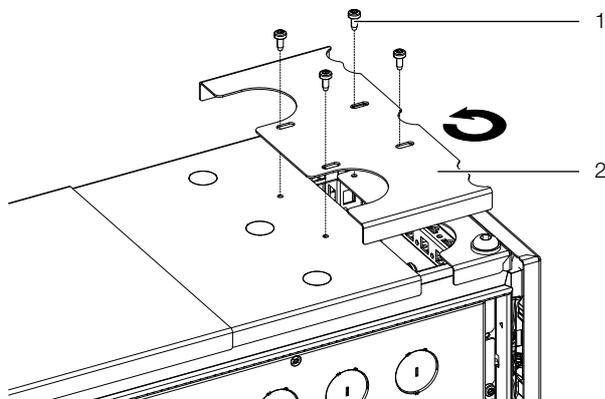
Fig. 81: Rotate the roof plate
