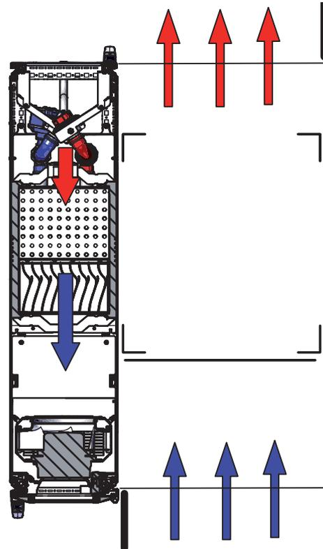
If the need arises, both the front and the rear door are automatically opened. The air flows unhindered into the interior of the enclosure, circulates around the installed equipment and exits the system via the open rear door of the enclosure. It is important to ensure that the LCP fans are switched off, otherwise hot air will be blasted in front of the 482.6 mm (19") level in the event of emergency cooling.
