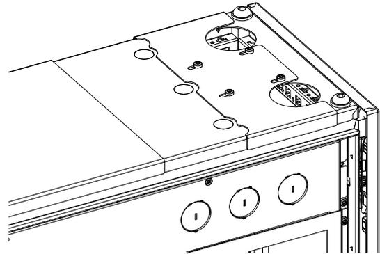
Fig. 82: Rotated roof plate
