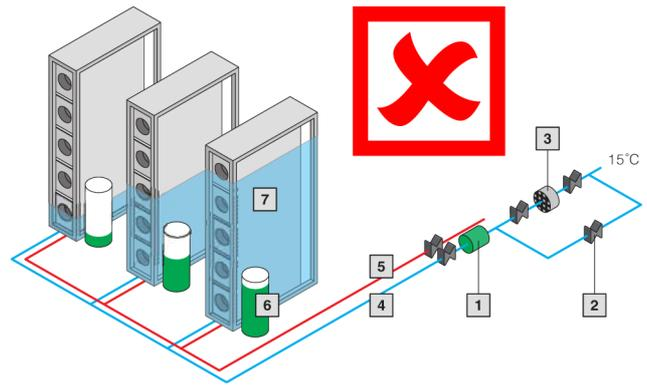
Fig. 84: Cooling distribution without hydraulic balancing
