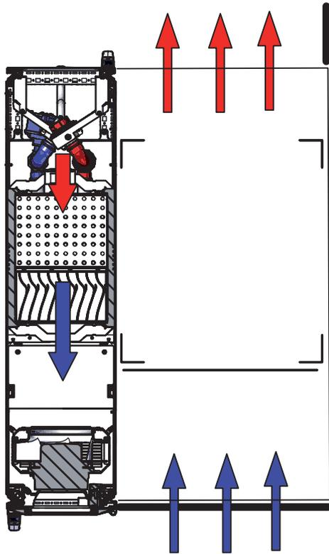
If the need arises, only the rear door of the enclosure is automatically opened. The air flows into the interior of the enclosure via the perforated front door, circulates around the installed equipment and exits the system via the open rear door of the enclosure. It is important to ensure that the LCP fans are switched off, otherwise hot air will be blasted in front of the 482.6 mm (19") level in the event of emergency cooling.
