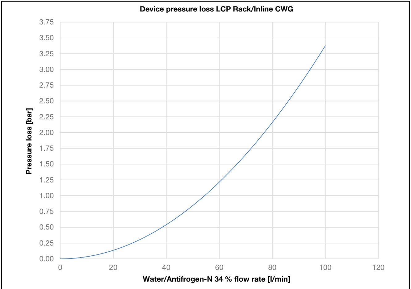
Fig. 125: Pressure loss of the LCP CWG
