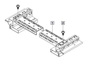
Punched rail 18 x 39 mm (mounting plate slide rail) 8617.700 - 8617.730
