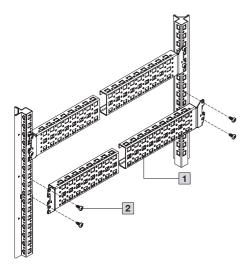
1 Punched section with mounting flange 8100.730 - 8100.733 8617.000 - 8617.060 8617.100 - 8617.210
