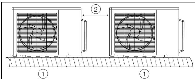
Fig. 8: Attachment points for external unit
