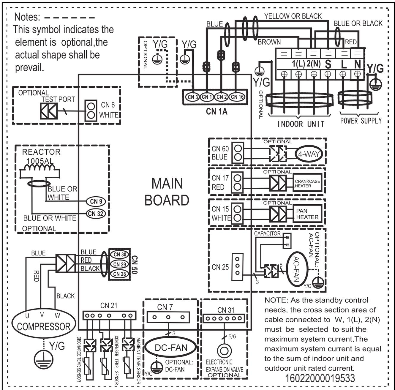
Fig. 27: Circuit diagram, external unit for 3 kW-devices (3311.490 and 3311.491)
