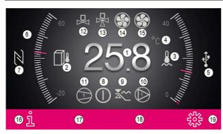
Fig. 14: Layout of the start screen
