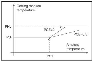
Fig. 17: Type of adjustment "relative with limit values"
