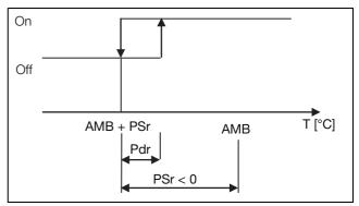
Fig. 18: Type of adjustment "relative with limit values"
