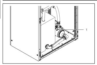
Fig. 13: Bleeding the cooling medium pump
