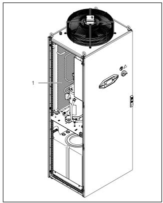
Fig. 23: Cleaning the condenser
