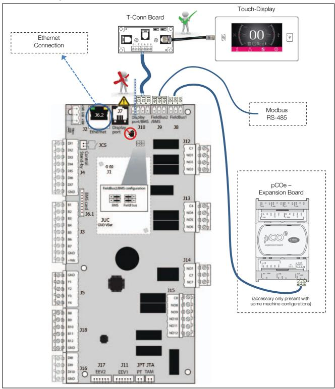
Fig. 34: Block diagram
