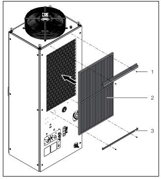
Fig. 11: Installing the metal filters
