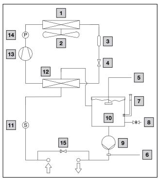
Fig. 3: Schematic diagram of refrigerant circuit (SK 33359x0)
