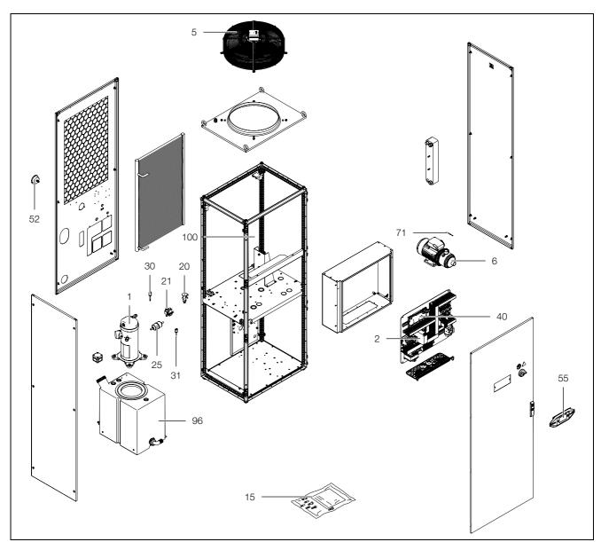
Fig. 35: Spare parts drawing
