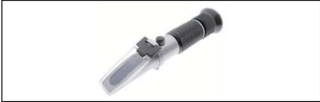
Fig. 22: Refractometer
