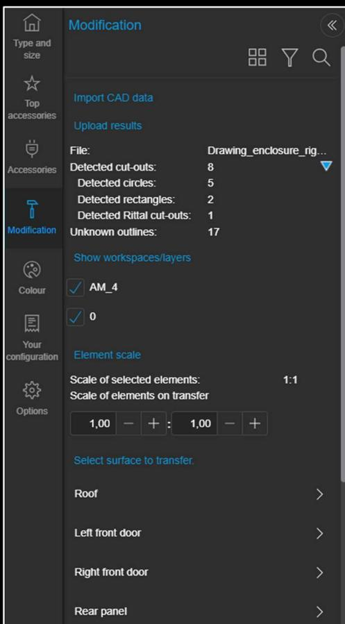
1. **Results** – all detected items such as circles are displayed in a bulleted list. The unknown and non-selectable geometries are also listed.
