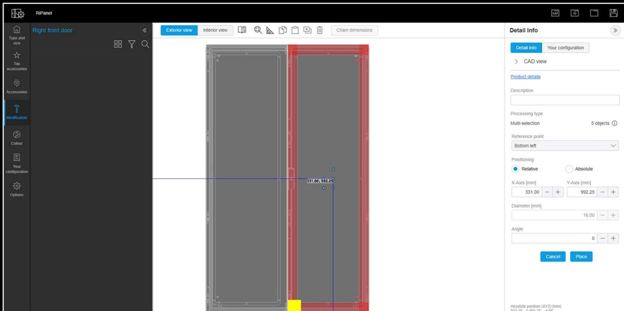
The reference geometry for the position can be selected by clicking on the desired geometry. You can identify the reference geometry by the reference lines. When your geometries are in the desired position, you can click the „Place“ button on the right side. Now it is also possible to move single geometries.
