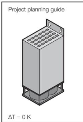
50 mm modules have 4 rows with openings in the ventilation grille
