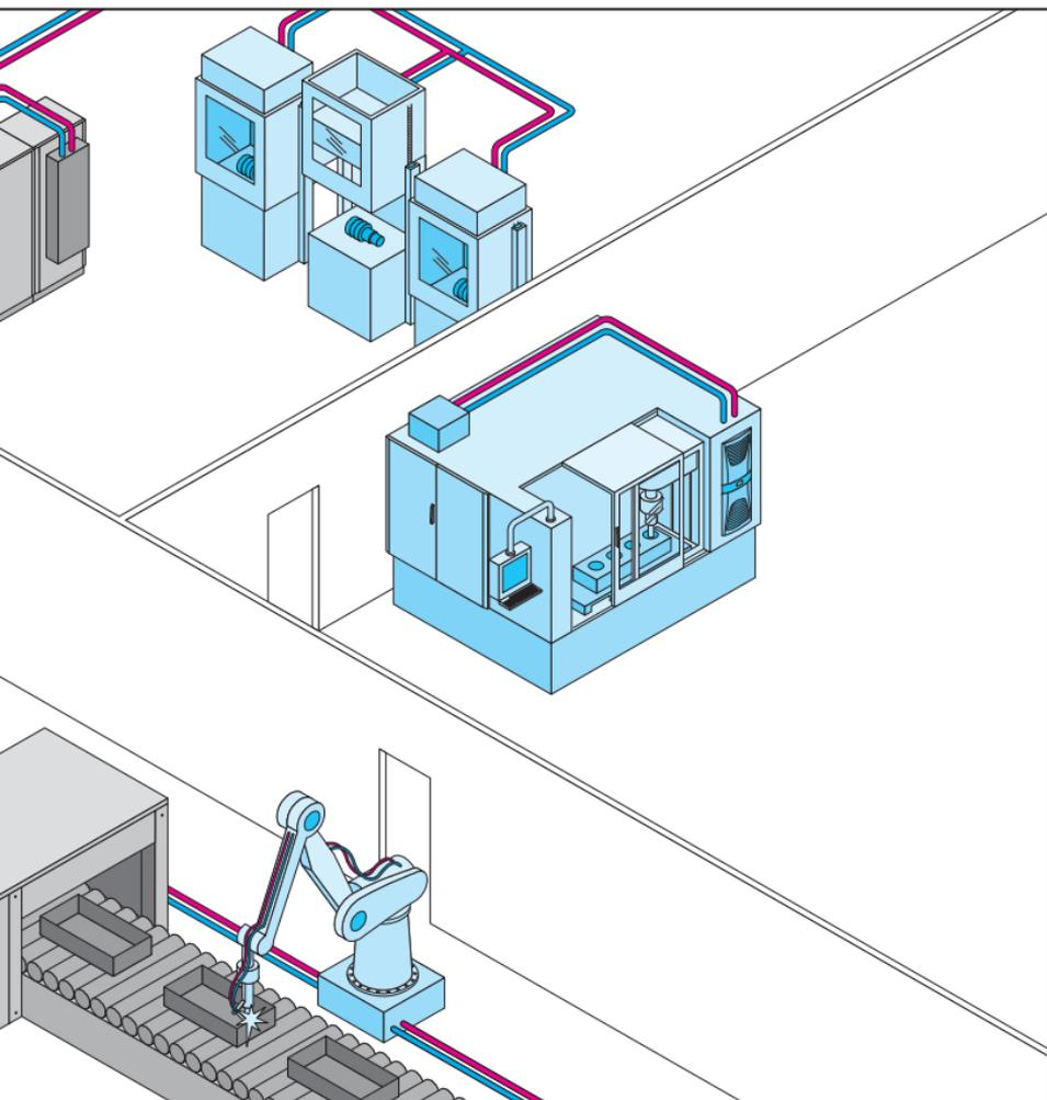
If a recooling system is intended to serve several pieces of equipment having different requirements in terms of the inlet temperature and flow rate of the cooling medium, e.g. combined machine and enclosure cooling, multi-circuit systems are used. With this solution, the different circuits
