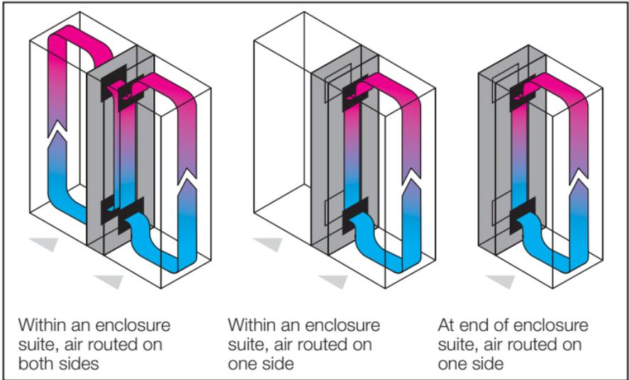
The advantage of these heat exchangers lies not only in the fact that a high cooling output can be achieved, but also that they can be fully and easily integrated into the Rittal TS 8 enclosure system.
