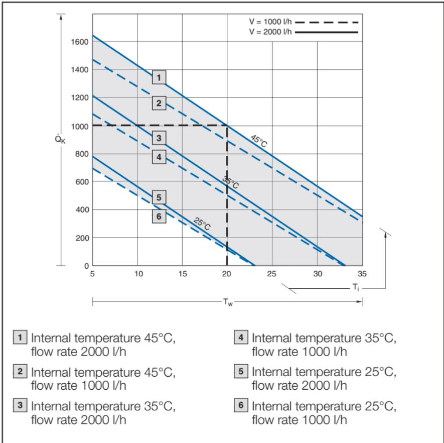
Here too, approx. 2000 l/h of cooling water is required. In particular it is worth noting the high energy efficiency of such a central solution for cooling whole suites of enclosures.
