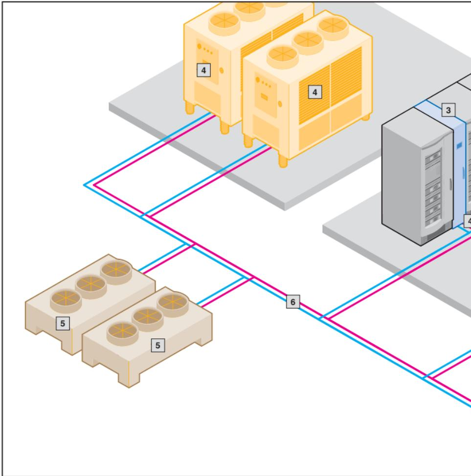
The cooling or air conditioning of a data centre is usually carried out using a raised floor, i.e. the air entering the data centre is cooled in an air-circulating climate control system (CRAC) and led to the room via the raised floor. The warm air from the
