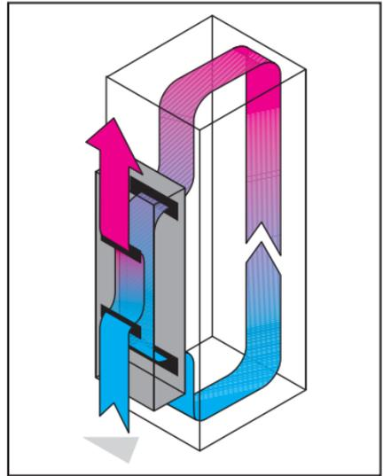
The operating principle is simple but very effective. The warm enclosure internal air is aspirated by a fan in the upper area and led through a cross-flow heat exchanger. The cooler ambient air is likewise aspirated by a fan and also led through this cross-flow heat exchanger, without the two air flows being mixed.
