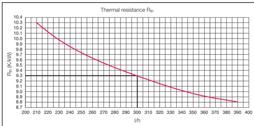
Characteristic of a water-cooled mounting plate (499 x 399 mm) with copper pipeline
