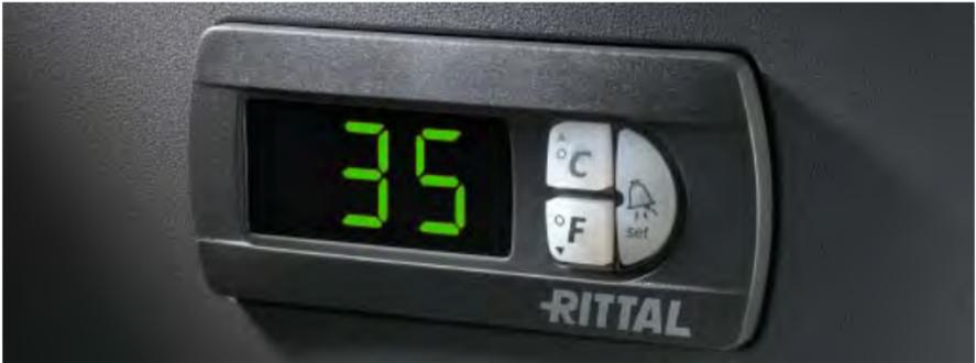
■ The internal temperature of the enclosure should always be set to +35°C. There is no technical justification for setting the temperature any lower. If the temperature inside the enclosure is lower than that, e.g. +15°C, condensation will be significantly increased.
