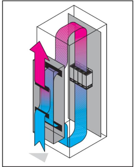
Electrical wires and cables are increasingly routed over the components. This inhibits the free dissipation of heat from these components to the ambient air in the enclosure.
