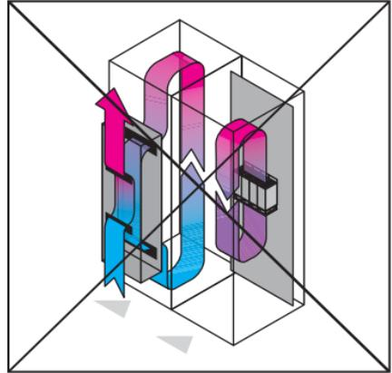
■ With all climate control solutions, the cold air should always be routed close to drive units (see illustration above). This is where the greatest heat losses occur. This arrangement ensures that the cold supply air from the climate control solution optimally cools the drive units without losses.
