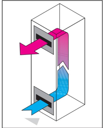
Innovative fan-and-filter units (with diagonal fan technology) with their novel design provide uniformly constant air throughput with optimised air routing and very low mounting depth, leaving more space in the enclosure compared with conventional axial fan-and-filter units.
