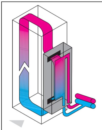
This requires a water connection (supply and return) and a central or decentralised cooling unit (recooler) for water cooling on the air/water heat exchanger. These heat exchangers are available for mounting on walls, installation in walls or roof mounting, depending on the application.
