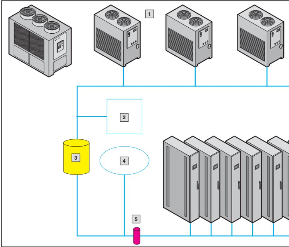
In addition, the use of “free cooling” ensures that the recooling systems, which are usually redundantly designed in the case of IT systems, are only used if the outdoor temperature exceeds the annual average of approx. 8.4°C, i.e. for about half the year. Through this technical solution, the system design actively helps reduce the energy costs of the data centre by a significant amount.
