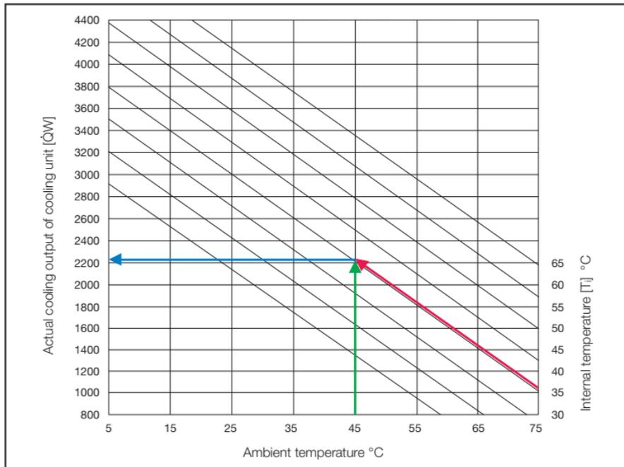
From the two reference variables of ambient temperature 45°C and enclosure internal temperature 35°C, one can determine the appropriate cooling unit (wall or roof-mounted) from a cooling performance diagram. Rittal has developed the “**Therm**” calculation program to simplify the design and calculation of enclosure cooling units and other climate control components.
