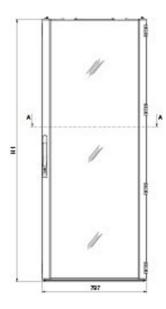
The TS IT rack stands out with its innovative solutions in enclosure roof and door designs. All doors are prepared for and assortment of locking options and come with 180°-hinges and comfort handles for both front and rear. Viewing doors are the first choice for rack climate control while perforated doors cater to room climate control – open ventilation accounts for 85% of the perforated area making previously unattainable air flow possible.
