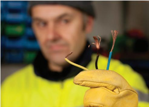
An arc flash is the explosive release of energy that occurs when there is a phase-to-phase or phase-to-ground arc fault. The many causes of an arc fault include: user error, accidental contact, corrosion, and insulation failure. Arc flash safety should be a major concern for any application that incorporates high current electrical equipment.
