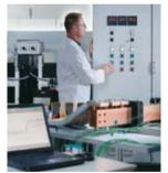
Verification of temperature rise is the most time-consuming verification, regardless of which method is used (testing, derivation or assessment). There are several methods to choose from, and these methods impose certain documentation requirements on the manufacturer.
