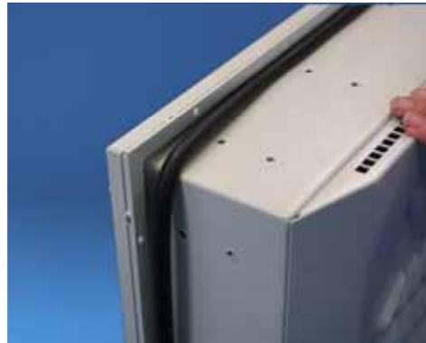
*Press the rubber seal into the mounting frame. Friction between the rubber seal and the enclosure is reduced due to the previous greasing. Additionally, the all-round rubber seal deforms more easily. This leads to optimum sealing when the device has been mounted.*
