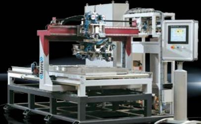
The wiring centre accelerates the wiring process by more than 400%, while at the same time minimising man hours. The patented machine head, which can be rotated through 270 degrees, lays the wires in the cable ducts and connects them to their respective components. Wires are replaced automatically, and can also be printed if required.
