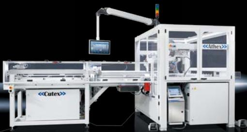
With this system, configuration with a wide range terminals from all well-known manufacturers is automated, accelerated and far more reliable. The generous magazine capacities of up to 40 terminal magazines help to minimise downtime and waiting time, while boosting flexibility. In conjunction with the Cutex (also available separately), prior to configuration the support rails are automatically fed from the magazines, cut to length and labelled.
