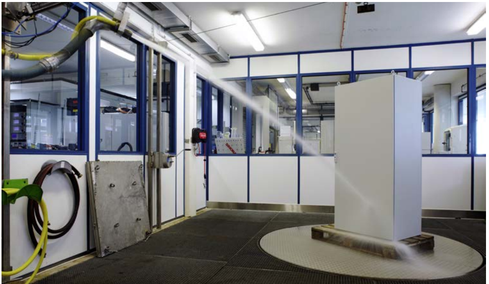
IP test in the Rittal test laboratory
