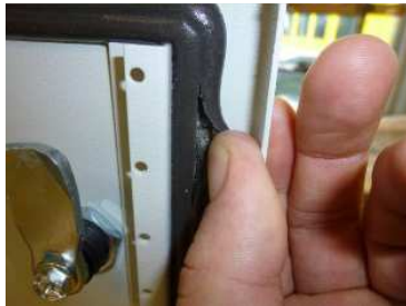
Image 4: Effects of an IK test
