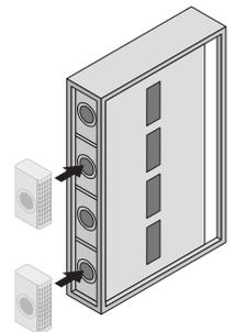
Adding two fans can increase cooling capacity to 30kw.
