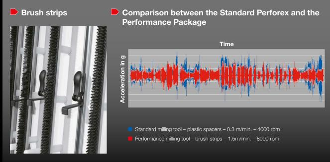
Brush strips provide a larger support area and ensure optimum vibration behaviour.
