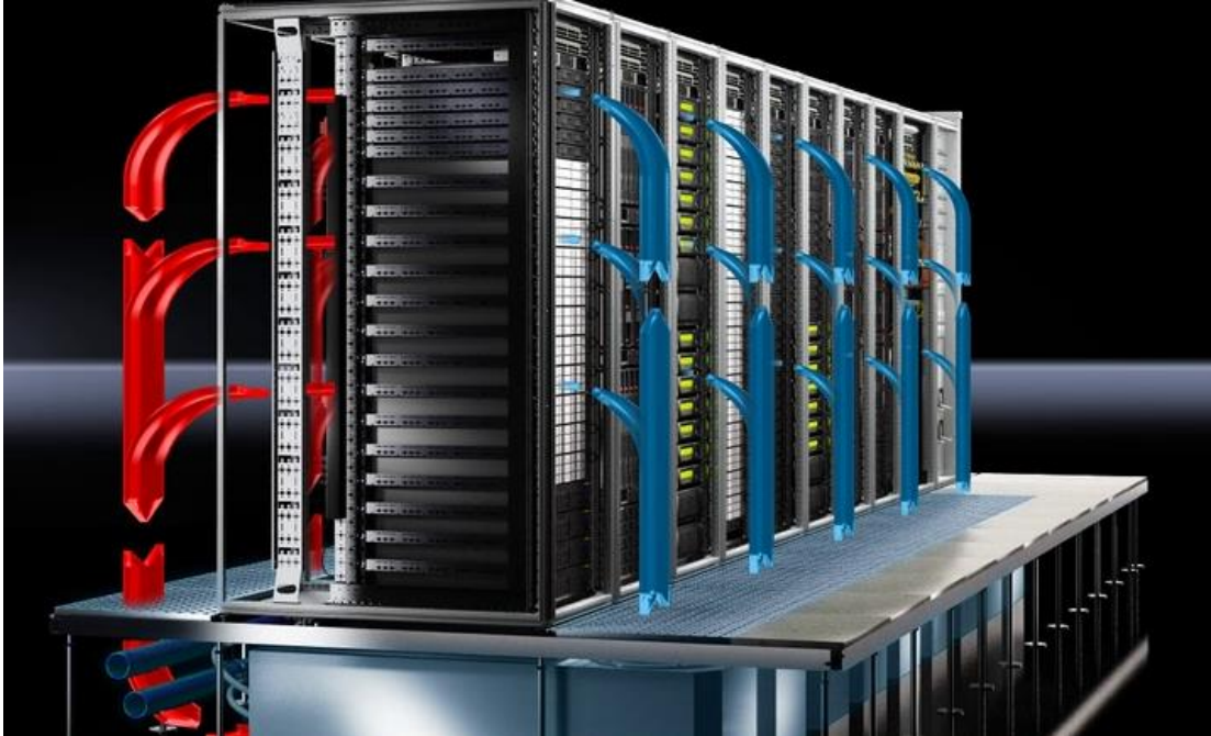
Figure 3: Air routing of the server modules
