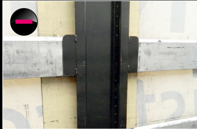
Protective packing on the stanchions. Undamaged inserts to prevent shipping damage caused by friction.
