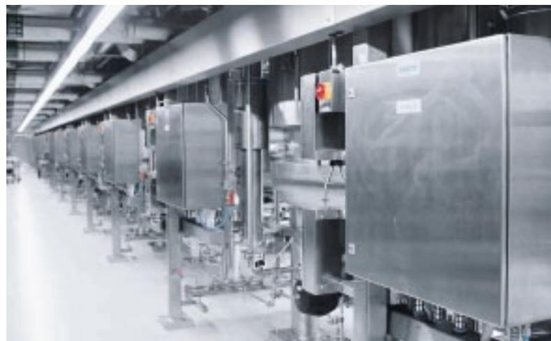
200 completely connection-ready stainless steel enclosures from Festo for the biotech factory’s 80 batch containers and bioreactors with some 5,000 valve functions approximately.
