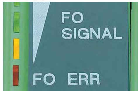
The four-level bar graph visualised the signal quality of the fibre optic path
