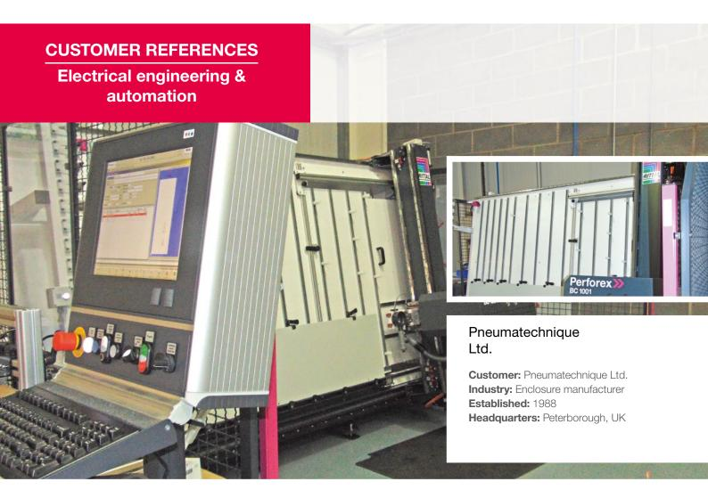
British enclosure constructor Pneumatechnique Ltd. was looking for ways to reduce its operating and overhead costs through automation. It found the solution it needed at Rittal Automation Systems: The Perforex machining centre reduces the machining time for enclosures, improves the accuracy of recurrent working operations, and allows specialist production staff to be deployed more efficiently.
