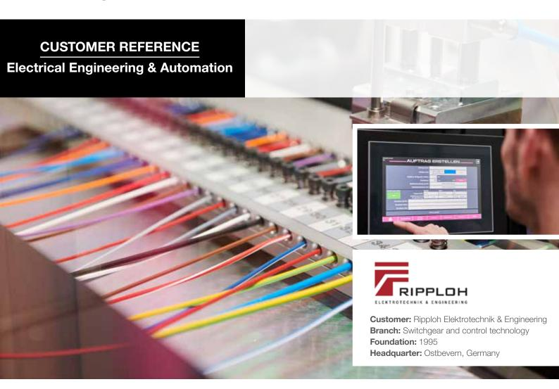
Promoting automation is Andreas Ripploh's goal. At his company, Ripploh Elektrotechnik & Engineering, for example, a Wire Terminal from Rittal is now in operation that significantly increases productivity in wire processing. The new machine can process as many as 1,500 wires during an eight-hour shift. And since there's no longer any need for operator intervention
