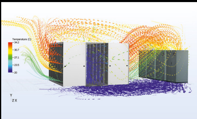
Airflow in a non-redundant enclosure with installed cold aisle containment.
