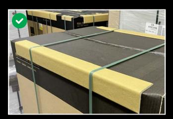
When using straps to secure loading units, use PET straps and edge protectors at its deflection points. The number of straps depends on the packing arrangement, total weight of all packaged products, and the location of the centre of gravity. We recommend using a minimum of two straps (crossed if need be).
