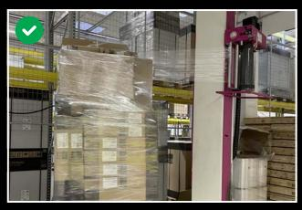
Only use a stretching machine or robot to stretch protective film around a load. Ensure that there is a transport- and handling-secure connection between the load and the load carrier, that the number of windings is sufficient and that the pre-load force is adequate.
