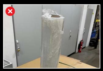
We would like to point out that wrapping the loading unit with wrapping film does not provide sufficient load securing when handling our goods.
