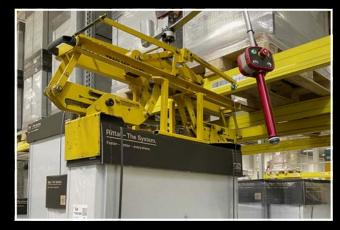
A suitable lifting tool can help to take pressure off of operating personnel.
