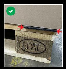
Non-slip materials, such as anti-slip mats or anti-slip paper, can be inserted between the load carrier and the load, and between the individual layers when goods are stacked, to keep load securing as straightforward as possible.
