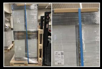
If necessary, the loading unit can also be stabilised and secured with a one-piece lashing strap and edge protectors.
