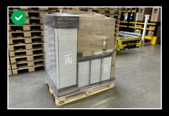
Avoid overhanging goods, gaps, cavities or empty spaces when forming mixed shipping units. Make sure that the upper layers of goods do not protrude beyond the lower layers. Ensure that the centre of gravity of the pallet is as central as possible and close to the load carrier.
