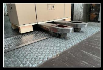
Ensure that the goods are standing securely. Always travel at an appropriately slow speed when driving over potential hazards and uneven surfaces.
