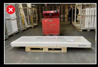
Never transport flat components on a smaller load carrier. These components could become deformed due to vibrations.
