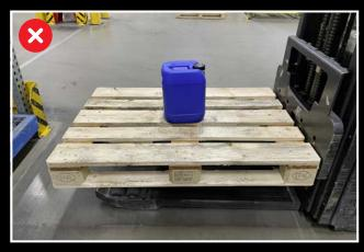
Never transport our canisters without additional load securing. These canisters could fall off and become damaged after a bend due to the surging movement of their contents.
