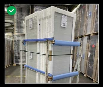
We therefore recommend that you cushion the goods at critical points to protect them from possible damage. The photo shows a possible example of this. It is also important to note that this type of product is particularly prone to tipping over during unloading.
