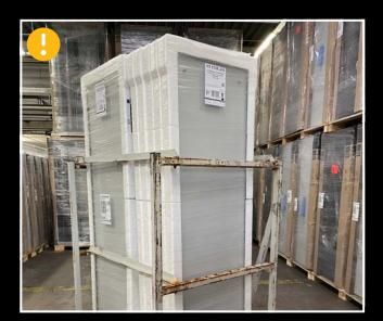
Special load carriers can be useful for the transport of flat components. It is important to note that friction between the product and the load carrier can cause damage to the goods.
