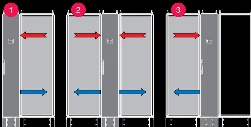
**1** At the beginning or end of a enclosure suite, air routing on one side
