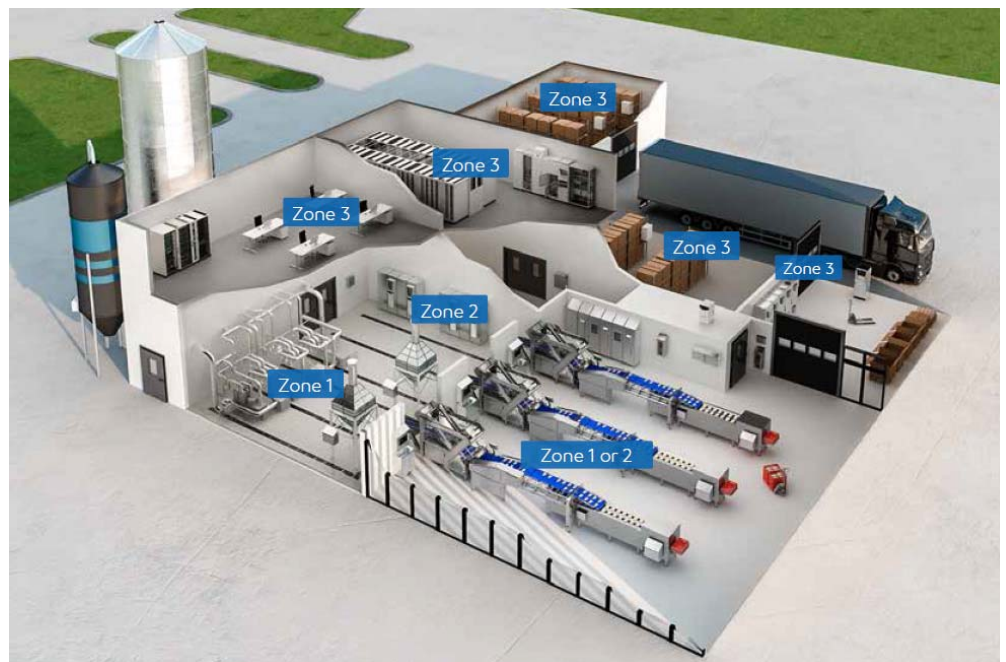
Figure 4: Schematic diagram of the hygiene zones at a company. There are three different types of goods. There are basically three different zones: These are the food zone (zone 1), the spray zone (zone 2) and the packaging and non-food zones (zone 3).
