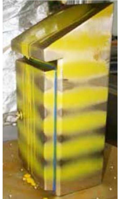
Figure 11: The contamination of the HD enclosure in the test.
