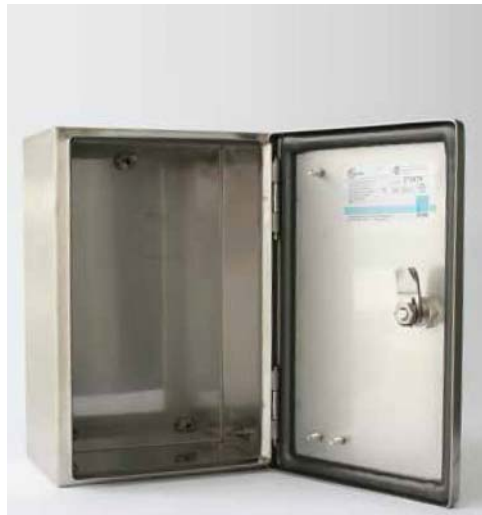
Figure 6: For example, the hinges are located outside the sealing area in an enclosure that is not of hygienic design.
