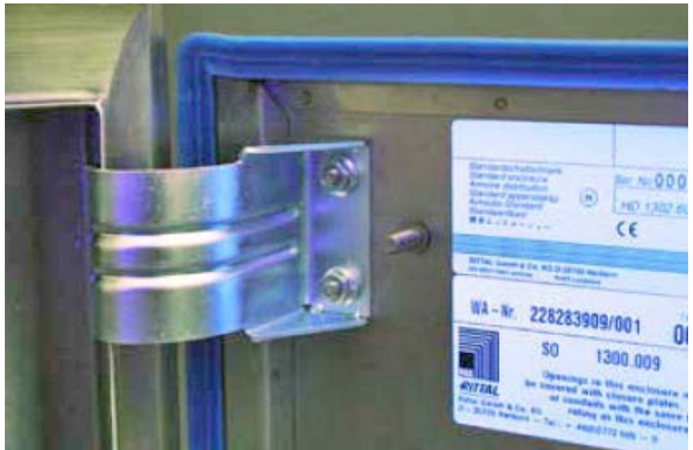
Figure 14: After the test has been performed on an HD enclosure, all the contamination is removed without leaving any residues.
