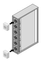
To achieve the max. cooling output of 60 kW, the customer/ service should install two additional fan modules
