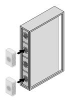
To achieve the max. cooling output of 30 kW, the customer/ service should install two additional fan modules.
